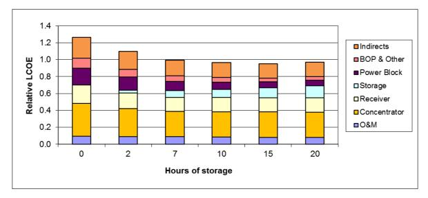
Figure C3: Modelling LCOE as a function of storage hours for a molten salt tower plant for Longreach Qld<sup>34</sup>.
