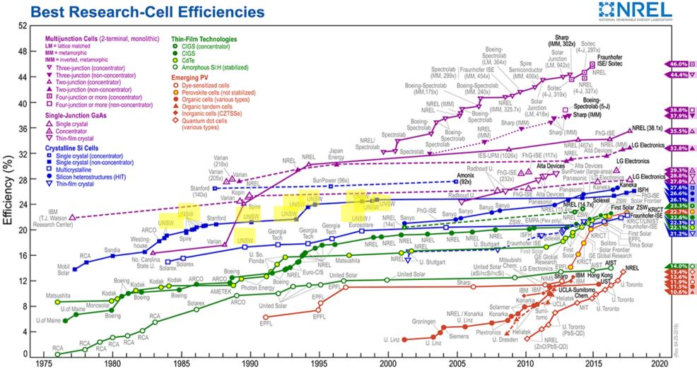
Figure 15: PV Cell types and efficiencies over time (NREL, 2018)<sup>12</sup>
